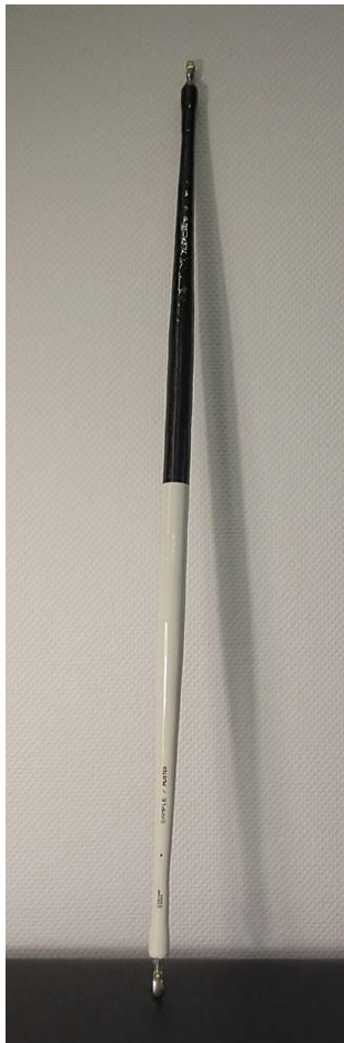
Figure 3: Composite Door Rod demonstrator manufactured by CirComp
